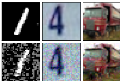
Fig. 3: (top) Clean image, (bottom) adversarial example for the maximum perturbation allowed (left to right: \epsilon = 0.4, 0.08, 0.04 ).
