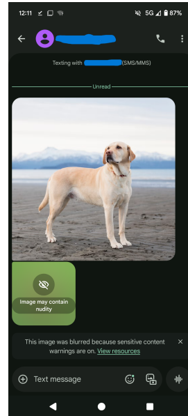
Fig. 1. User interface of the Google Messages application with SafetyCore enabled. When nudity is detected by the AI model, the image is blurred and a warning message is displayed to the user.
